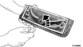
3. Pull bulb straight from socket to remove.
